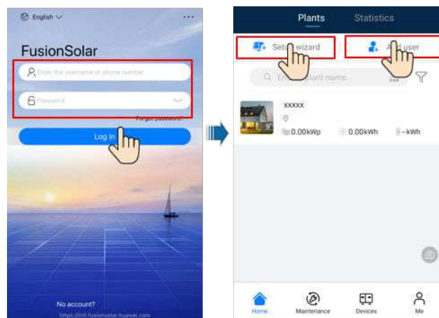
Figure 7-3 Creating a PV plant and a user
